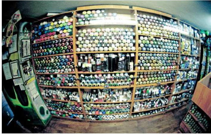
Figure 4.21: An image with barrel distortion, taken by a fish-eyed lens. (Image by Wikipedia user Ilveon.)
