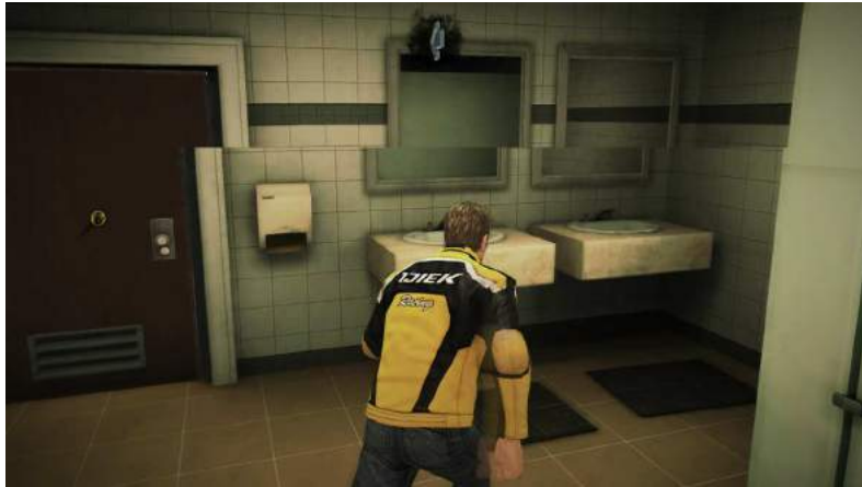
Figure 7.17: If a new frame is written to the video memory while a display scanout occurs, then tearing arises, in which parts of two or more frames become visible at the same time. (Figure from http://www.overclock.net/ user Forceman.)
