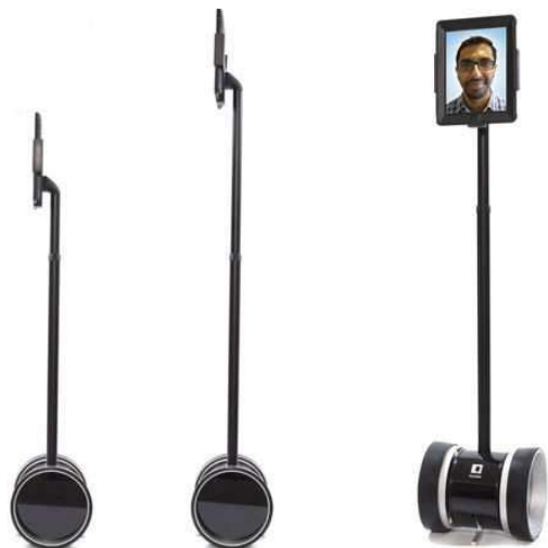
Figure 13.9: The Double telepresence robot is a screen and camera on a stick. The robot costs around $2500, and the screen is a tablet, such as an iPad. The height can even be adjusted remotely so that the person may appear to be sitting or standing. (Picture by Double Robotics.)
