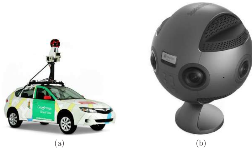
Figure 1.9: An important component for achieving telepresence is to capture a panoramic view: (a) A car with cameras and depth sensors on top, used by Google to make Street View. (b) The Insta360 Pro captures and streams omnidirectional videos.
