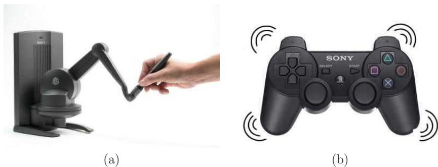
Figure 2.8: Two examples of haptic feedback devices. (a) The Touch X system by 3D Systems allows the user to feel strong resistance when poking into a virtual object with a real stylus. A robot arm provides the appropriate forces. (b) Some game controllers occasionally vibrate.
