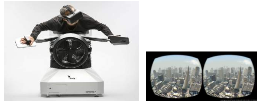
Figure 1.1: In the Birdly experience from the Zurich University of the Arts, the user, wearing a VR headset, flaps his wings while flying over virtual San Francisco. A motion platform and fan provide additional sensory stimulation. The figure on the right shows the stimulus presented to each eye.
