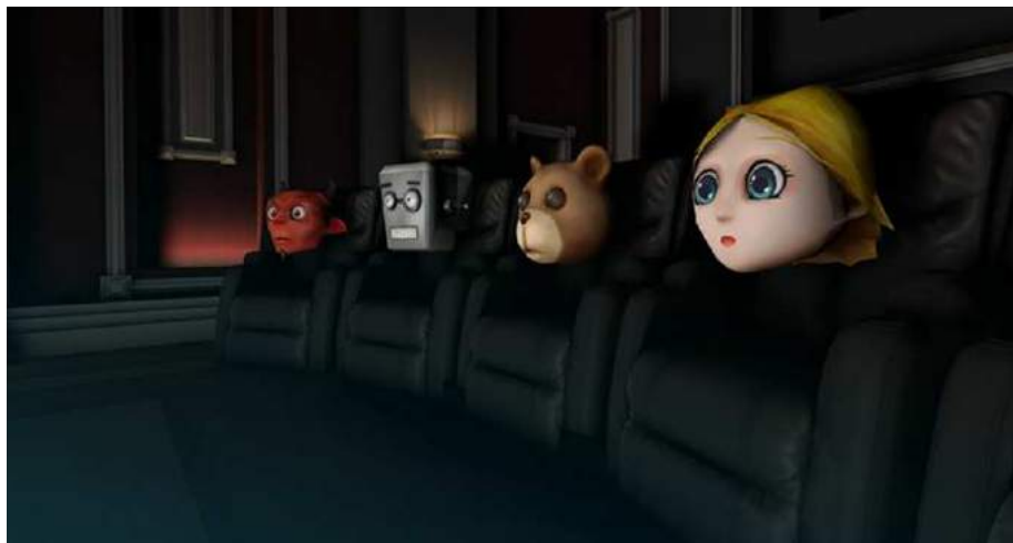
Figure 10.17: Oculus Social Alpha, which was an application for Samsung Gear VR. Multiple users could meet in a virtual world and socialize. In this case, they are watching a movie together in a theater. Their head movements are provided using head tracking data. They are also able to talk to each other with localized audio.
