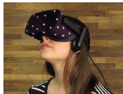
Figure 9.13: The Oculus Rift headset contains IR LEDs hidden behind IR-transparent plastic. (Photo from www.ifixit.com .)
