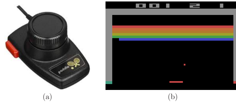
Figure 10.2: (a) Atari 2600 Paddle controller. (b) The Atari Breakout game, in which the bottom line segment is a virtual paddle that allows the ball to bounce to the top and eliminate bricks upon contacts.
