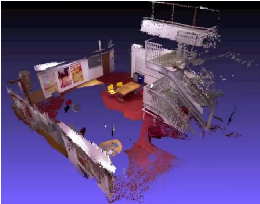
Figure 2.14: Using both color and depth information from cameras, a 3D model of the world can be extracted automatically using Simultaneous Localization and Mapping (SLAM) techniques. Figure from [130].
